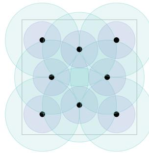
Then these larger spheres have to cover the entire space — since if there were some uncovered point, then we could have added a sphere at that point to the original packing.
